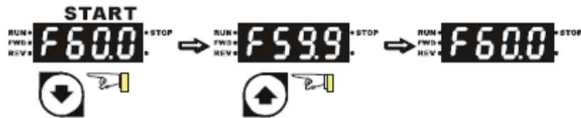
**Setting direction** (When operation source is digital keypad)
